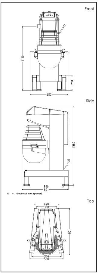
Electric Supply voltage: 200-240 V/1N ph/50/60 Hz Electrical power, max: 2.2 kW Total Watts: 2.2 kW
